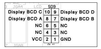
When used with a non-alphanumeric display, shifter positions will be indicated as "1" through "9" with Neutral being displayed as "0" and Reverse as a blank output. These outputs can be used to drive a 7-segment display through any standard BCD-TO-SEVEN SEGMENT decoder driver chip as illustrated bellow.
