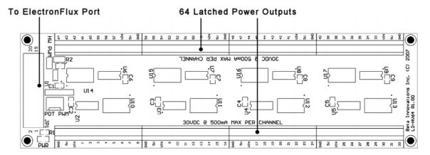
The LO-HV64 card is a passive device and will not be automatically detected by your USB module. You will need to activate the port of your module and set it to Latched Output mode in the Device Manager utility in order to use the LO-HV64 outputs.
