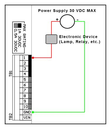
Multiple electronic devices such as lamps can be connected to the same channel provided the total current does not exceed max ratings for that channel.
