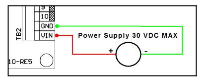
IMPORTANT: Any external power supply used with the DO10-RE5 card on channels 1 to 10 must be tied to VIN and GND terminals on TB2 as illustrated above. Failure to do so may cause irreparable damage to the card and will void the product warranty.
