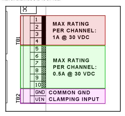
In additional to isolating high voltage, high current loads from the IO port, clamping input on VIN provides additional protection when used with inductive loads.
