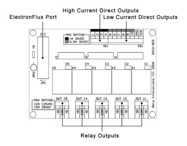
The DO10-RE5 card is a passive device and will not be automatically detected by your USB module. You will need to activate the port of your module and set it to Direct Output mode in the Device Manager utility in order to use the DO10-RE5 outputs.
